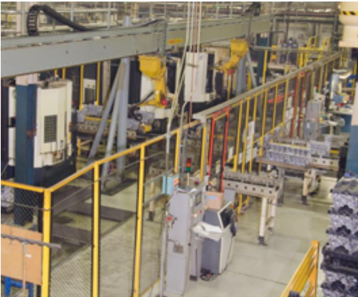
GANTRY ROBOT CELL FOR REPEATABLE VOLUME PRODUCTION.
