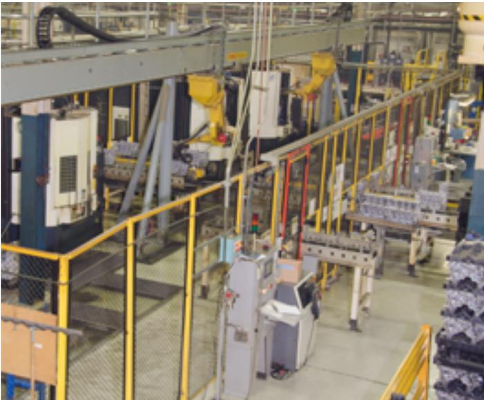
GANTRY ROBOT CELL FOR REPEATABLE VOLUME PRODUCTION.
