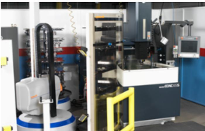
ROBOT-TENDED SINKER EDM CELL WITH AUTOMATED LOAD/UNLOAD OF TOOLING AND WORKPIECES.
