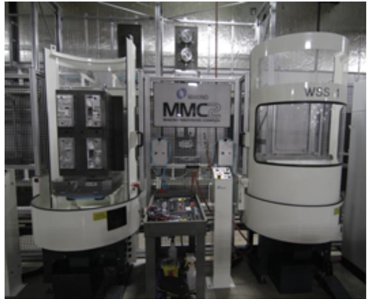
MMC2 FLEXIBLE MANUFACTURING SYSTEM FOR 24/7 MACHINING.
