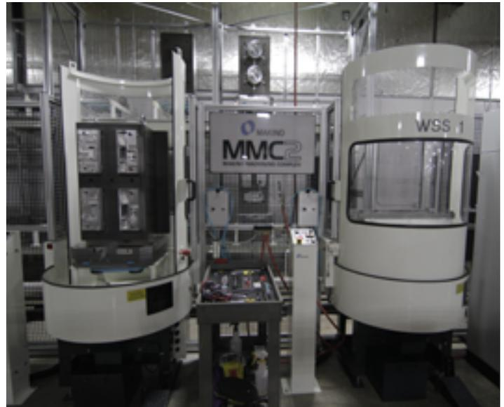
MMC2 FLEXIBLE MANUFACTURING SYSTEM FOR 24/7 MACHINING.
