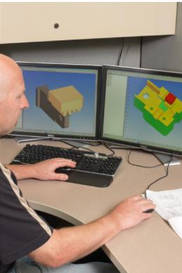
Program all machines (especially sinker EDM) offline to enhance machine uptime and to reinforce the practice of creating NC programs and performing toolpath simulation away from the physical machine tool.
