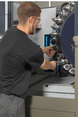
Use your current automated tool changer (ATC). Become accustomed to using your ATC for unattended operation, if you have not already. Set up your tool magazines with redundant tooling, and make sure your operators are confident in using and relying upon current machine and control functions that facilitate automatic operations.
