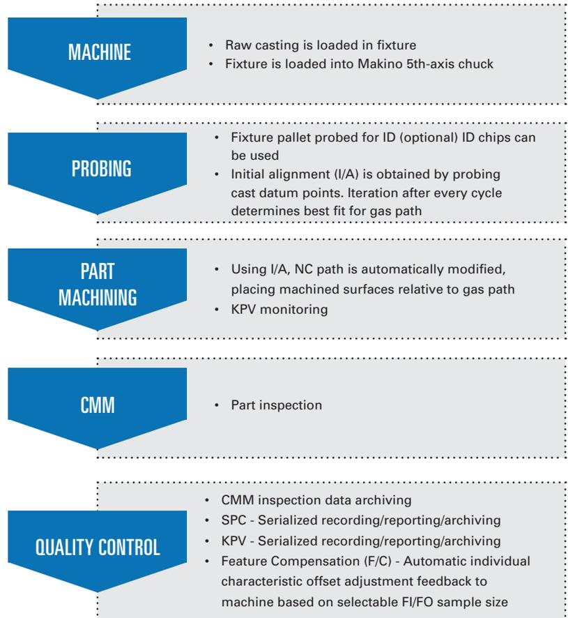
on how often the part has been in the spindle and how accurate it is. The KPV data is usually kept for each part so that the manufacturer can go back later and look at how a part was produced.
