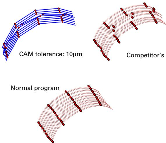
Less capable NC controller software simply executes the code as presented. Even with multiline read ahead, the result is a choppy surface that requires additional post process work in polishing or deburring to generate the desired finish. How much cost is wrapped up in unoptimized finishing and hand work, due in part to poor finishes from the milling operation?
